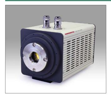
The C12741-11 is a near-infrared camera which employs a 640 × 512 pixel InGaAs sensor. -70 °C peltier cooling significantly reduces dark current which leads to improved image quality and allows imaging with long exposure time.
