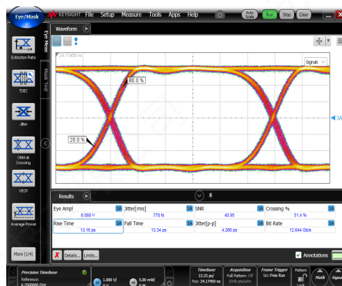
Output response Eye amplitude = 6\text{ V}_{pp}
