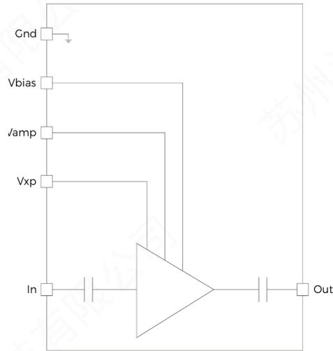
Mechanical Diagram and Pinout
