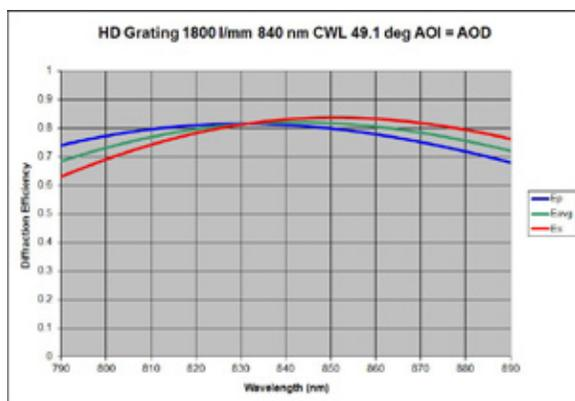
We measure every transmissive VPH grating to ensure exceptional 1<sup>st</sup> order diffraction efficiency uniformity over the specified operating band. Not all vendors do!
